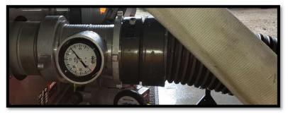
Air and water temperature for all testing remained in the mid-60's degree Fahrenheit range. Elevation was approximately 900 feet ASL. For each flow rate on each strainer tested, pump discharge pressure was maintained at 150psi. Once the throttle and valves were set and readings had stabilized, readings were taken at zero, one minute, and two minutes.
